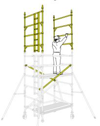
Add two more diagonal braces between the 5th and 7th rungs. If finishing at this height (4.2m platform), reposition the fixed deck to the 8th rung on the tower. Fit a trapdoor deck alongside it, with the hinges towards the outside of the tower, and the trapdoor next to the ladder. Add a single diagonal between the 7th and 9th rungs as shown. Climb up the ladder, and from the protected trapdoor position, fit the guardrails on the 9th and 10th rungs, in that order, on both sides of the tower.
